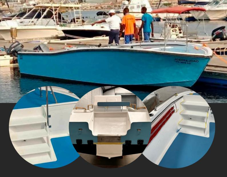
The Skye Goods Transporter 8500 is built for rugged reliability, ensuring safe and efficient transport of local goods, produce, and fish across diverse marine environments. Its rubberized, non-slip deck enhances stability and protection, minimizing the risk of slips and falls while ensuring secure footing during loading, transit, and unloading operations.
